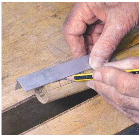
▲ Pic. 5 Using a strip of angle as a saddle gauge to run the centre line down the leg
